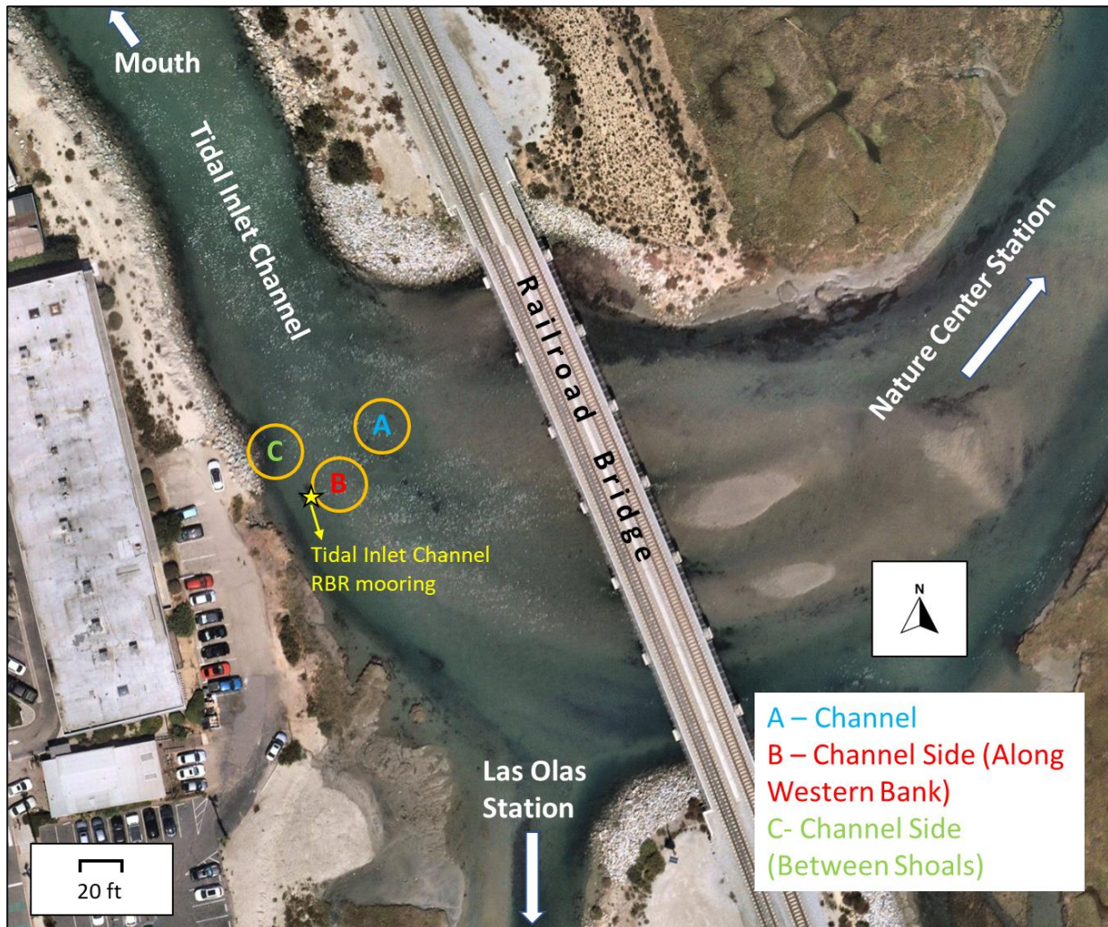
Figure 3-5: Map of 2022 Aquadopp deployment locations at the Tidal Inlet Channel.
