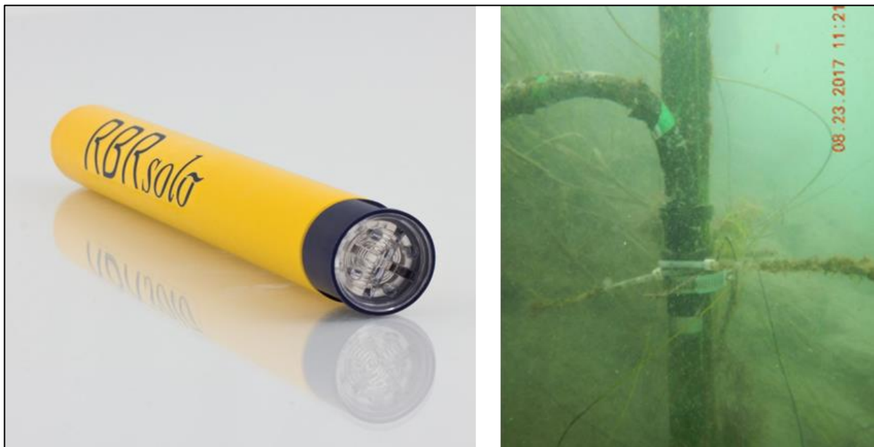
Figure 2-2: RBR Solo D tide gauge for water level measurements (left) and an example of the mounting system (right) during the 2017 deployment.
